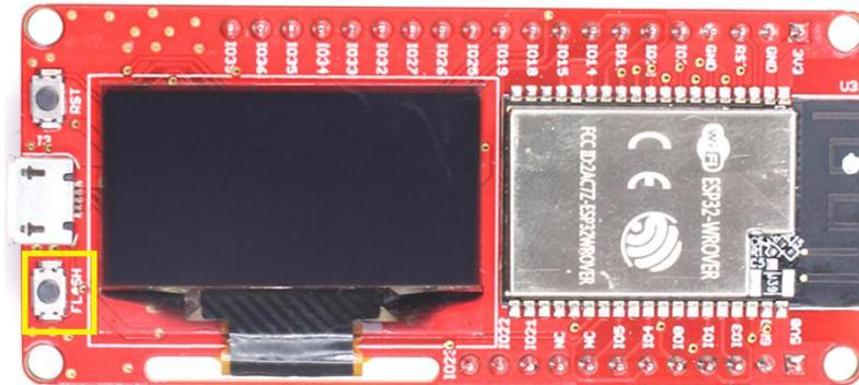
While holding down the “FLASH”, click the “ok” button in the burn firmware window:
