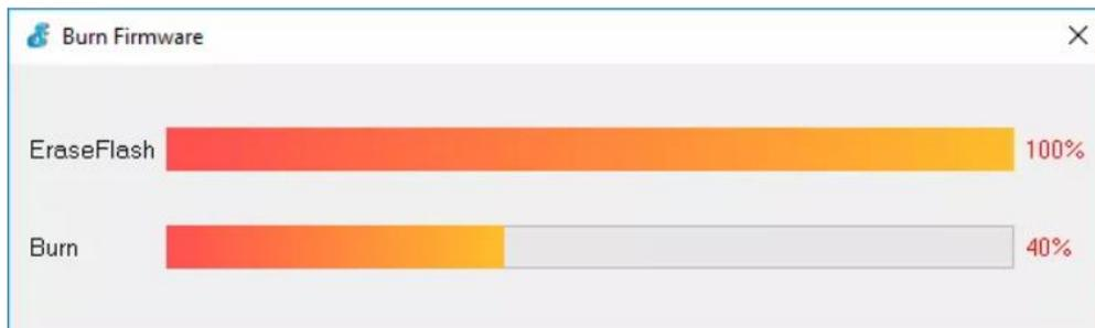
**\*Note:** if the “EraseFlash” bar doesn’t move and you see an error message saying “erase false.”, it means that your ESP32 wasn’t in flashing mode. You need to repeat all the steps described earlier and hold the “FLASH” button again to ensure that your ESP32 goes into flashing mode.
