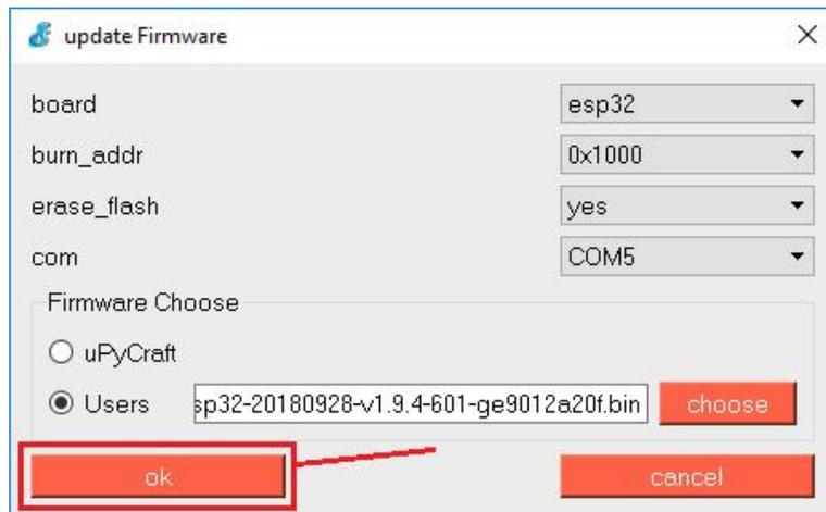
When the “EraseFlash” process begins, you can release the “FLASH” button. After a few seconds, the firmware will be flashed into your ESP32 board.
